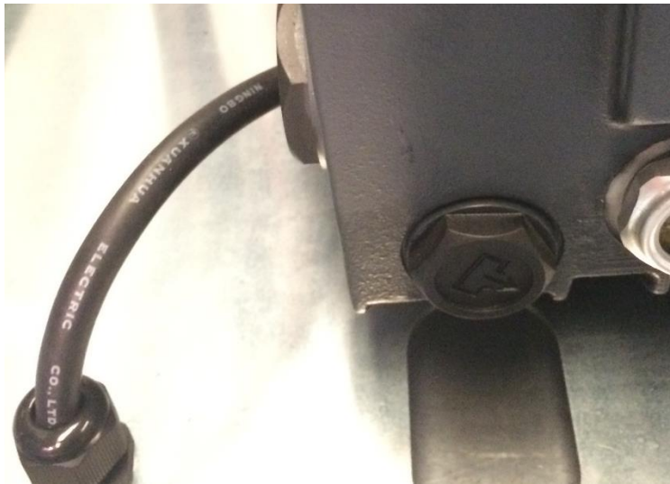
Illustration 5. Remove the oil drainage plug
