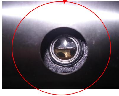
Illustration 1. Rear display for checking the oil level
