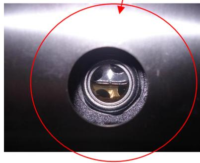
**Illustration 1. Rear display for checking the oil level**
