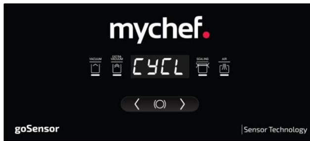
**Figure 6. Vacuum cycles completed view**
