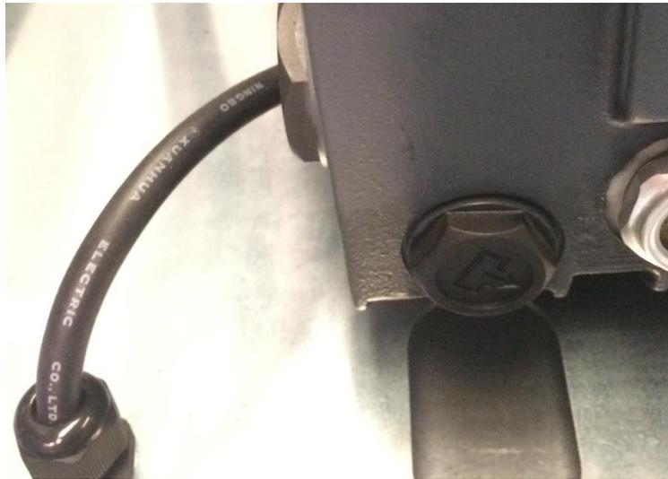
**Illustration 5. Remove the oil drainage plug**
