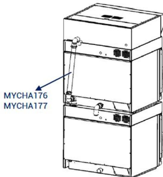
**Figure 4. Hood connection in stacked ovens**
