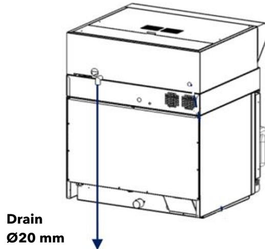
**Figure 3. Drain connection**
