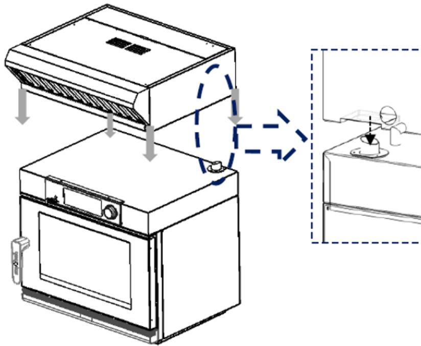
**Figure 1. Positioning of the condensation hood**
