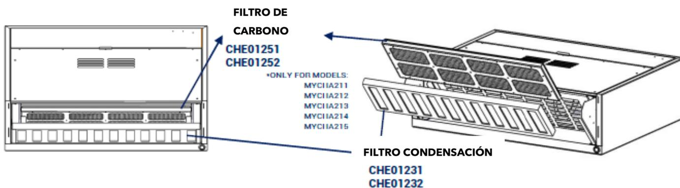
**Figure 8. Removal of condensation filter and carbon filter**
