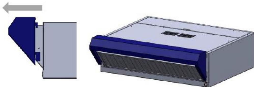
**Figure 7. Front cover removal**
